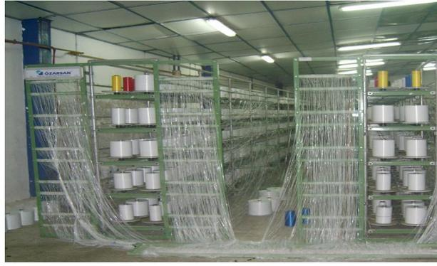
1400 Vertical spinning coil adapter and tension mechanism, big bag for warping creels. So wound coils are used for.
